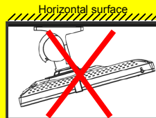
*Ceiling mount or mount on any other horizontal surface overhead are not advisable
